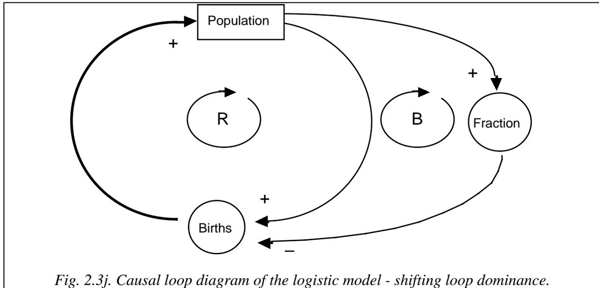
Fig. 2.3j. Causal loop diagram of the logistic model - shifting loop dominance.
